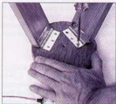
Pre-drilling the screw-holes for the hinges will make attaching the legs much easier.
