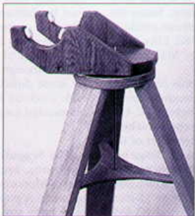
Cradle box attached. Note the tension triangle wedge placed to keep legs spread.
