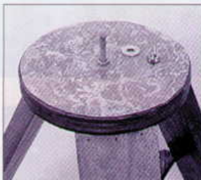
The bottom board with a 1/4"-20 bolt protruding to fit into the cradle box
