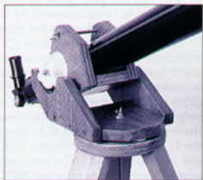
The scope held securely in the side-bearing box fits neatly inside the cradle box.
