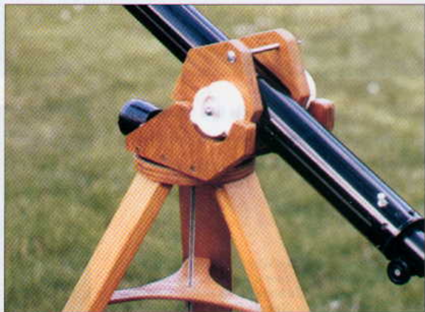
The finished mount with telescope loaded and ready to use. Add a small counterweight to the front of the cradle box if needed for better balance.
