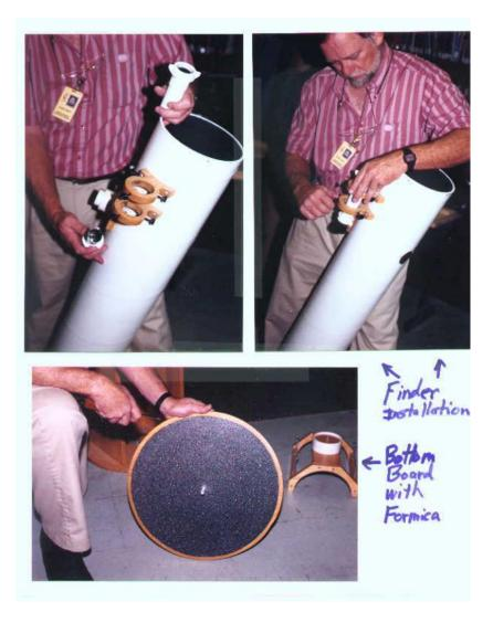
The ground board and the base board must have teflon in contact with Formica or some other brand of plastic laminate. Rough surface Formica works best. Get some teflon pads at the hardware store in the chair leg section. The ground board is the one closest to the ground. It will have some stubby feet at three points where it contacts the ground.
