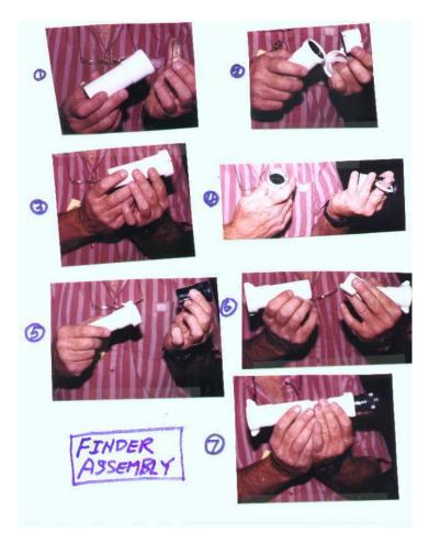
Once you have a 35mm binocular objective, get a 1.5" plastic drain tube extension and a 1.25" plastic drain tube extension. The 35mm lens should slide into the 1.5 inch adapter and stop where
